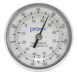
ProSense bi-metal dial thermometer, 3in diameter, 4in insertion length, -40 to 160 deg F/-40 to 70 deg C, 1/2in male NPT process connection, center back mount.
