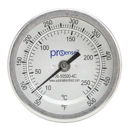
ProSense bi-metal dial thermometer, 3in diameter, 4in insertion length, 50 to 500 deg F/10 to 260 deg C, 1/2in male NPT process connection, center back mount.
