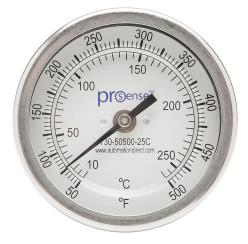
ProSense bi-metal dial thermometer, 3in diameter, 2-1/2in insertion length, 50 to 500 deg F/10 to 260 deg C, 1/2in male NPT process connection, center back mount.
