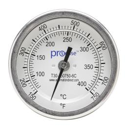
ProSense bi-metal dial thermometer, 3in diameter, 6in insertion length, 150 to 750 deg F/70 to 400 deg C, 1/2in male NPT process connection, center back mount.
