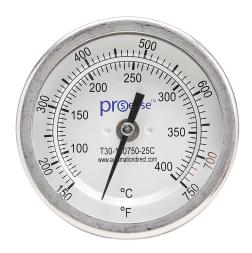
ProSense bi-metal dial thermometer, 3in diameter, 2-1/2in insertion length, 150 to 750 deg F/70 to 400 deg C, 1/2in male NPT process connection, center back mount.
