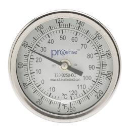
ProSense bi-metal dial thermometer, 3in diameter, 6in insertion length, 0 to 250 deg F/-18 to 120 deg C, 1/2in male NPT process connection, center back mount.
