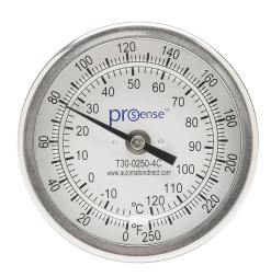
ProSense bi-metal dial thermometer, 3in diameter, 4in insertion length, 0 to 250 deg F/-18 to 120 deg C, 1/2in male NPT process connection, center back mount.
