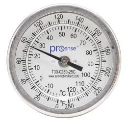
ProSense bi-metal dial thermometer, 3in diameter, 2 1/2in insertion length, 0 to 250 deg F/-18 to 120 deg C, 1/2in male NPT process connection, center back mount.
