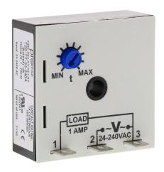
ProSense on-interval relay timer, 1 to 100 minutes timing range, 24-240 VAC operating voltage, 1A contact rating, (1) SPNO timed solid state relay output(s), surface mount, 1/4in male quick-connect terminal.
