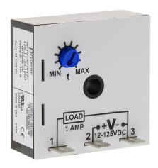
ProSense on-interval relay timer, 1 to 100 minutes timing range, 12-125 VDC operating voltage, 1A contact rating, (1) SPNO timed solid state relay output(s), surface mount, 1/4in male quick-connect terminal.
