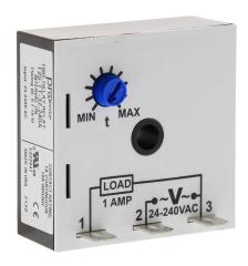
ProSense on-interval relay timer, 0.1 to 10 minutes timing range, 24-240 VAC operating voltage, 1A contact rating, (1) SPNO timed solid state relay output(s), surface mount, 1/4in male quick-connect terminal.
