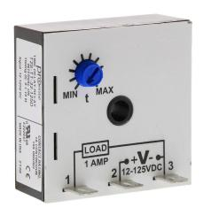
ProSense on-interval relay timer, 0.1 to 10 minutes timing range, 12-125 VDC operating voltage, 1A contact rating, (1) SPNO timed solid state relay output(s), surface mount, 1/4in male quick-connect terminal.
