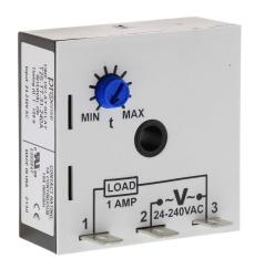
ProSense on-interval relay timer, 1 to 100 seconds timing range, 24-240 VAC operating voltage, 1A contact rating, (1) SPNO timed solid state relay output(s), surface mount, 1/4in male quick-connect terminal.
