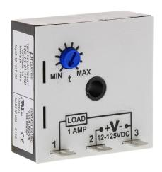
ProSense on-interval relay timer, 1 to 100 seconds timing range, 12-125 VDC operating voltage, 1A contact rating, (1) SPNO timed solid state relay output(s), surface mount, 1/4in male quick-connect terminal.
