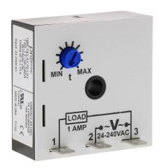
ProSense on-interval relay timer, 0.1 to 10 seconds timing range, 24-240 VAC operating voltage, 1A contact rating, (1) SPNO timed solid state relay output(s), surface mount, 1/4in male quick-connect terminal.
