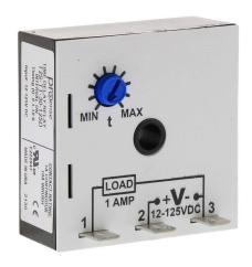
ProSense on-interval relay timer, 0.1 to 10 seconds timing range, 12-125 VDC operating voltage, 1A contact rating, (1) SPNO timed solid state relay output(s), surface mount, 1/4in male quick-connect terminal.
