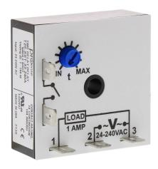
ProSense fleeting (single-shot) relay timer, 1 to 100 minutes timing range, 24-240 VAC operating voltage, 1A contact rating, (1) SPNO timed solid state relay output(s), surface mount, 1/4in male quick-connect terminal.
