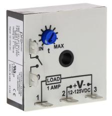
ProSense fleeting (single-shot) relay timer, 1 to 100 minutes timing range, 12-125 VDC operating voltage, 1A contact rating, (1) SPNO timed solid state relay output(s), surface mount, 1/4in male quick-connect terminal.
