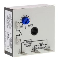
ProSense fleeting (single-shot) relay timer, 0.1 to 10 minutes timing range, 24-240 VAC operating voltage, 1A contact rating, (1) SPNO timed solid state relay output(s), surface mount, 1/4in male quick-connect terminal.
