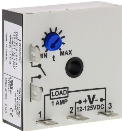
ProSense fleeting (single-shot) relay timer, 0.1 to 10 minutes timing range, 12-125 VDC operating voltage, 1A contact rating, (1) SPNO timed solid state relay output(s), surface mount, 1/4in male quick-connect terminal.
