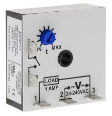
ProSense fleeting (single-shot) relay timer, 1 to 100 seconds timing range, 24-240 VAC operating voltage, 1A contact rating, (1) SPNO timed solid state relay output(s), surface mount, 1/4in male quick-connect terminal.
