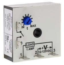
ProSense fleeting (single-shot) relay timer, 1 to 100 seconds timing range, 12-125 VDC operating voltage, 1A contact rating, (1) SPNO timed solid state relay output(s), surface mount, 1/4in male quick-connect terminal.
