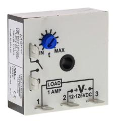
ProSense fleeting (single-shot) relay timer, 1 to 100 seconds timing range, 12-125 VDC operating voltage, 1A contact rating, (1) SPNO timed solid state relay output(s), surface mount, 1/4in male quick-connect terminal.
