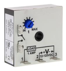
ProSense fleeting (single-shot) relay timer, 0.1 to 10 seconds timing range, 12-125 VDC operating voltage, 1A contact rating, (1) SPNO timed solid state relay output(s), surface mount, 1/4in male quick-connect terminal.
