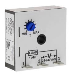
ProSense on-delay relay timer, 1 to 100 minutes timing range, 24-240 VAC operating voltage, 1A contact rating, (1) SPNO timed solid state relay output(s), surface mount, 1/4in male quick-connect terminal.
