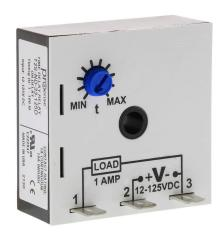
ProSense on-delay relay timer, 1 to 100 minutes timing range, 12-125 VDC operating voltage, 1A contact rating, (1) SPNO timed solid state relay output(s), surface mount, 1/4in male quick-connect terminal.
