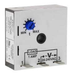
ProSense on-delay relay timer, 0.1 to 10 minutes timing range, 24-240 VAC operating voltage, 1A contact rating, (1) SPNO timed solid state relay output(s), surface mount, 1/4in male quick-connect terminal.
