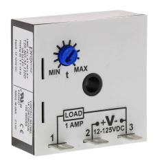
ProSense on-delay relay timer, 0.1 to 10 minutes timing range, 12-125 VDC operating voltage, 1A contact rating, (1) SPNO timed solid state relay output(s), surface mount, 1/4in male quick-connect terminal.
