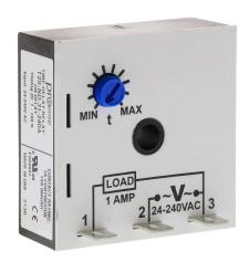
ProSense on-delay relay timer, 1 to 100 seconds timing range, 24-240 VAC operating voltage, 1A contact rating, (1) SPNO timed solid state relay output(s), surface mount, 1/4in male quick-connect terminal.
