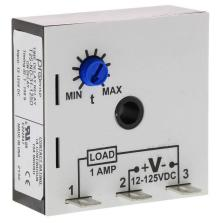
ProSense on-delay relay timer, 1 to 100 seconds timing range, 12-125 VDC operating voltage, 1A contact rating, (1) SPNO timed solid state relay output(s), surface mount, 1/4in male quick-connect terminal.
