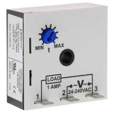
ProSense on-delay relay timer, 0.1 to 10 seconds timing range, 24-240 VAC operating voltage, 1A contact rating, (1) SPNO timed solid state relay output(s), surface mount, 1/4in male quick-connect terminal.
