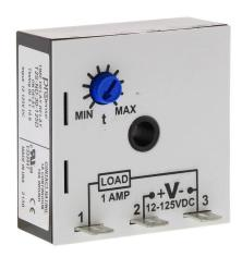
ProSense on-delay relay timer, 0.1 to 10 seconds timing range, 12-125 VDC operating voltage, 1A contact rating, (1) SPNO timed solid state relay output(s), surface mount, 1/4in male quick-connect terminal.
