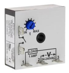
ProSense off-delay relay timer, 1 to 100 minutes timing range, 24-240 VAC operating voltage, 1A contact rating, (1) SPNO timed solid state relay output(s), surface mount, 1/4in male quick-connect terminal.
