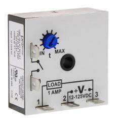
ProSense off-delay relay timer, 0.1 to 10 minutes timing range, 12-125 VDC operating voltage, 1A contact rating, (1) SPNO timed solid state relay output(s), surface mount, 1/4in male quick-connect terminal.
