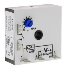
ProSense off-delay relay timer, 1 to 100 seconds timing range, 24-240 VAC operating voltage, 1A contact rating, (1) SPNO timed solid state relay output(s), surface mount, 1/4in male quick-connect terminal.
