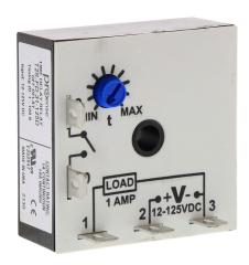
ProSense off-delay relay timer, 1 to 100 seconds timing range, 12-125 VDC operating voltage, 1A contact rating, (1) SPNO timed solid state relay output(s), surface mount, 1/4in male quick-connect terminal.
