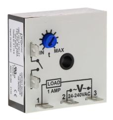
ProSense off-delay relay timer, 0.1 to 10 seconds timing range, 24-240 VAC operating voltage, 1A contact rating, (1) SPNO timed solid state relay output(s), surface mount, 1/4in male quick-connect terminal.
