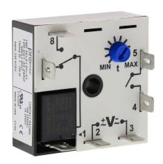
ProSense fleeting (single-shot) relay timer, 1 to 100 minutes timing range, 24 VAC/VDC operating voltage, 10A contact rating, (1) SPDT timed relay output(s), surface mount, 1/4in male quick-connect terminal.
