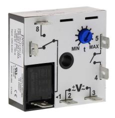
ProSense fleeting (single-shot) relay timer, 1 to 100 minutes timing range, 120 VAC/VDC operating voltage, 10A contact rating, (1) SPDT timed relay output(s), surface mount, 1/4in male quick-connect terminal.
