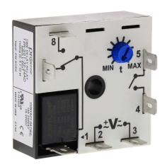
ProSense fleeting (single-shot) relay timer, 0.1 to 10 minutes timing range, 24 VAC/VDC operating voltage, 10A contact rating, (1) SPDT timed relay output(s), surface mount, 1/4in male quick-connect terminal.
