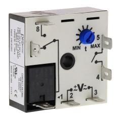
ProSense fleeting (single-shot) relay timer, 1 to 100 seconds timing range, 24 VAC/VDC operating voltage, 10A contact rating, (1) SPDT timed relay output(s), surface mount, 1/4in male quick-connect terminal.
