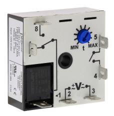
ProSense fleeting (single-shot) relay timer, 1 to 100 seconds timing range, 120 VAC/VDC operating voltage, 10A contact rating, (1) SPDT timed relay output(s), surface mount, 1/4in male quick-connect terminal.
