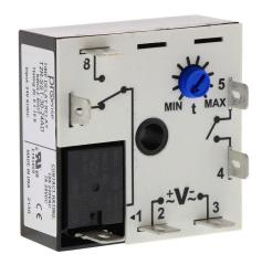
ProSense fleeting (single-shot) relay timer, 0.1 to 10 seconds timing range, 24 VAC/VDC operating voltage, 10A contact rating, (1) SPDT timed relay output(s), surface mount, 1/4in male quick-connect terminal.
