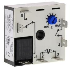
ProSense fleeting (single-shot) relay timer, 0.1 to 10 seconds timing range, 120 VAC/VDC operating voltage, 10A contact rating, (1) SPDT timed relay output(s), surface mount, 1/4in male quick-connect terminal.
