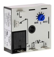
ProSense on-delay relay timer, 1 to 100 minutes timing range, 24 VAC/VDC operating voltage, 10A contact rating, (1) SPDT timed relay output(s), surface mount, 1/4in male quick-connect terminal.
