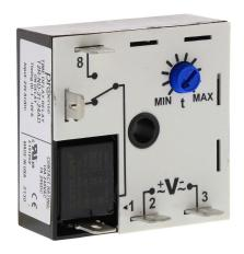
ProSense on-delay relay timer, 1 to 100 seconds timing range, 24 VAC/VDC operating voltage, 10A contact rating, (1) SPDT timed relay output(s), surface mount, 1/4in male quick-connect terminal.
