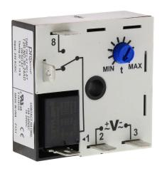
ProSense on-delay relay timer, 0.1 to 10 seconds timing range, 24 VAC/VDC operating voltage, 10A contact rating, (1) SPDT timed relay output(s), surface mount, 1/4in male quick-connect terminal.
