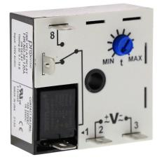
ProSense on-delay relay timer, 0.1 to 10 seconds timing range, 120 VAC/VDC operating voltage, 10A contact rating, (1) SPDT timed relay output(s), surface mount, 1/4in male quick-connect terminal.
