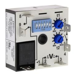
ProSense multi-mode relay timer, 0.1 seconds to 1,000 minutes selectable timing range, 24-240 VAC and 12-125 VDC operating voltage, 10A contact rating, (1) SPDT timed relay output(s), surface mount, 1/4in male quick-connect terminal.
