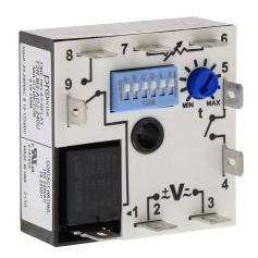
ProSense multi-mode relay timer, 0.1 seconds to 100 minutes selectable timing range, 24-240 VAC and 12-125 VDC operating voltage, 10A contact rating, (1) SPDT timed relay output(s), surface mount, 1/4in male quick-connect terminal.
