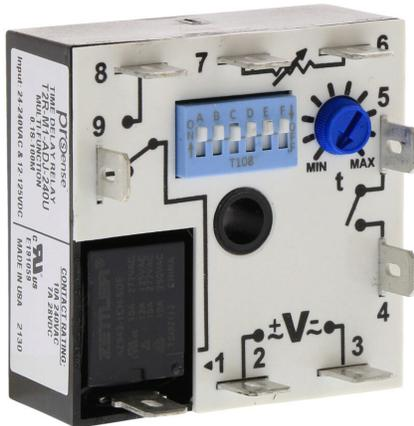
ProSense multi-mode relay timer, 0.1 seconds to 100 minutes selectable timing range, 24-240 VAC and 12-125 VDC operating voltage, 10A contact rating, (1) SPDT timed relay output(s), surface mount, 1/4in male quick-connect terminal.
